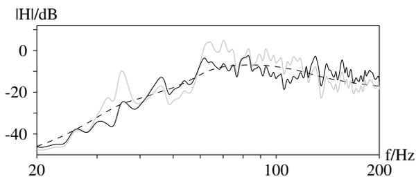
Figure 12:  $H_{max}$  (gray),  $H_t$  (dashed), and equalized curve  $H_{eqd}$  (black) of the basement.
