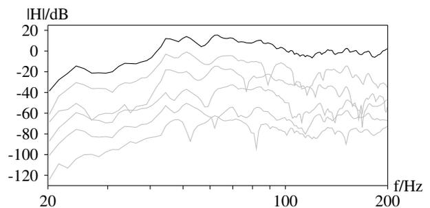
Figure 6: Room responses (gray) separated with 15 dB offsets for better visibility and the resulting maximum norm  $H_{max}$  (black).
