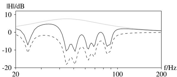
Figure 9: Equalization curve (dashed), bass loss compensation curve (gray), and combined curve (black).
