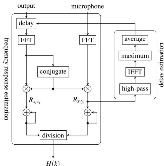
Figure 2: The dual channel FFT analysis method with automatic synchronization.
