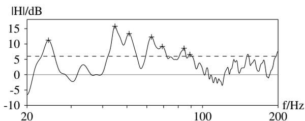
Figure 8: Compensated response (solid) and detection threshold (dashed). The detected peaks in the range from 20 to 120 Hz are marked by a +.
