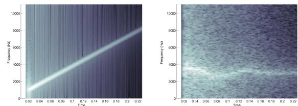
Figure 2: Spectrograms of the basic sound events employed: bubble (on the left) and impact (on the right)
